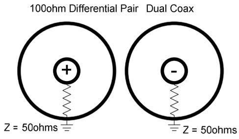
Of course, this simple case of “pure delay difference” could be fixed by inserting a matching “pure delay” in the signal path of the shorter of the two cables. This may be easy in concept, but is not a solution for the general case.
