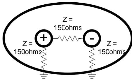
Any imbalance in the differential pair, such as asymmetry of length or twist or dielectric environment, results in some intra-pair skew.
