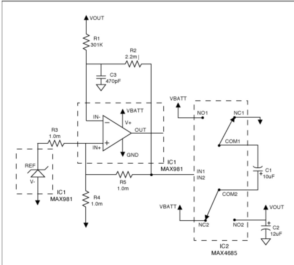
Figure 1. Low-Iq regulated charge pump.
