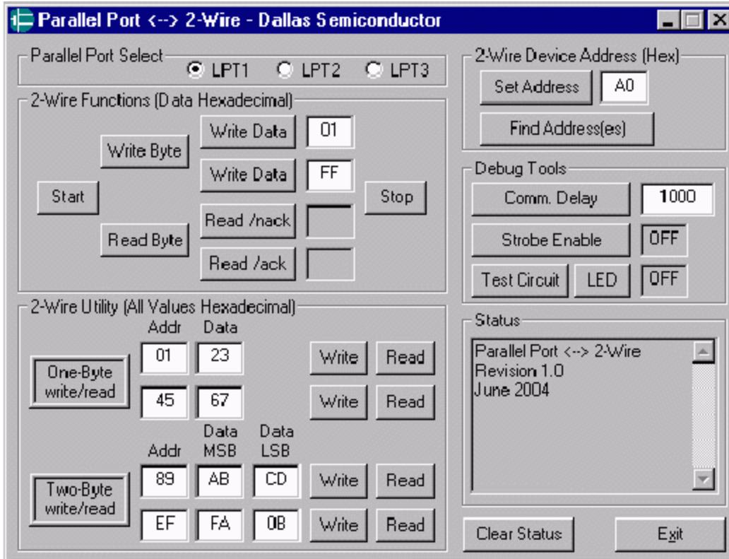
Figure 1. Example Windows parallel port to 2-Wire software.
