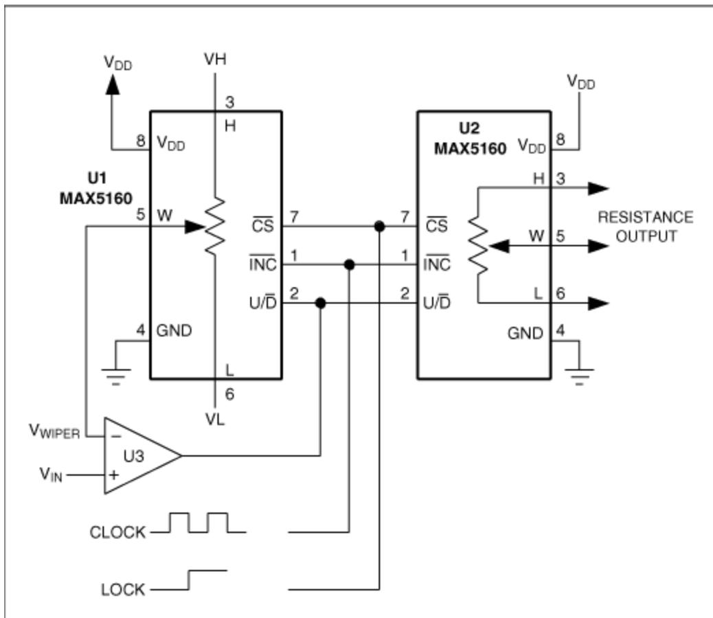
Figure 1. Two identical digital potentiometers enable this circuit to implement voltage-to-resistance
