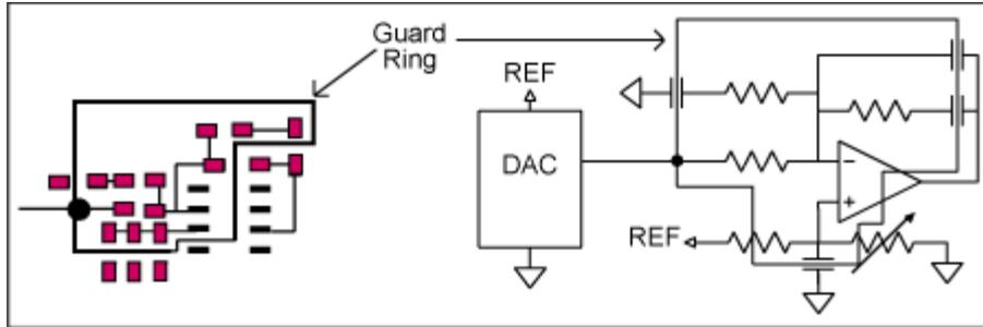
Figure 2. PCB layout for guard ring.
