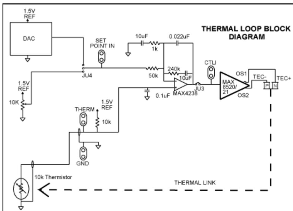
Figure 1. Block diagram for thermal control loop.
