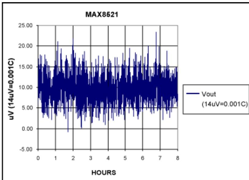
Figure 6. Long term Stability Plot (Maximum error 0.0018°C).
