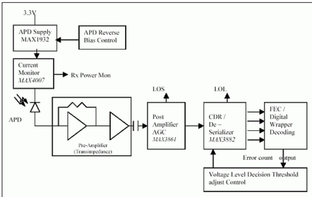
Figure 3a. Example of a 2.5Gbps DWDM receiver with linear preamplifier and AGC.
