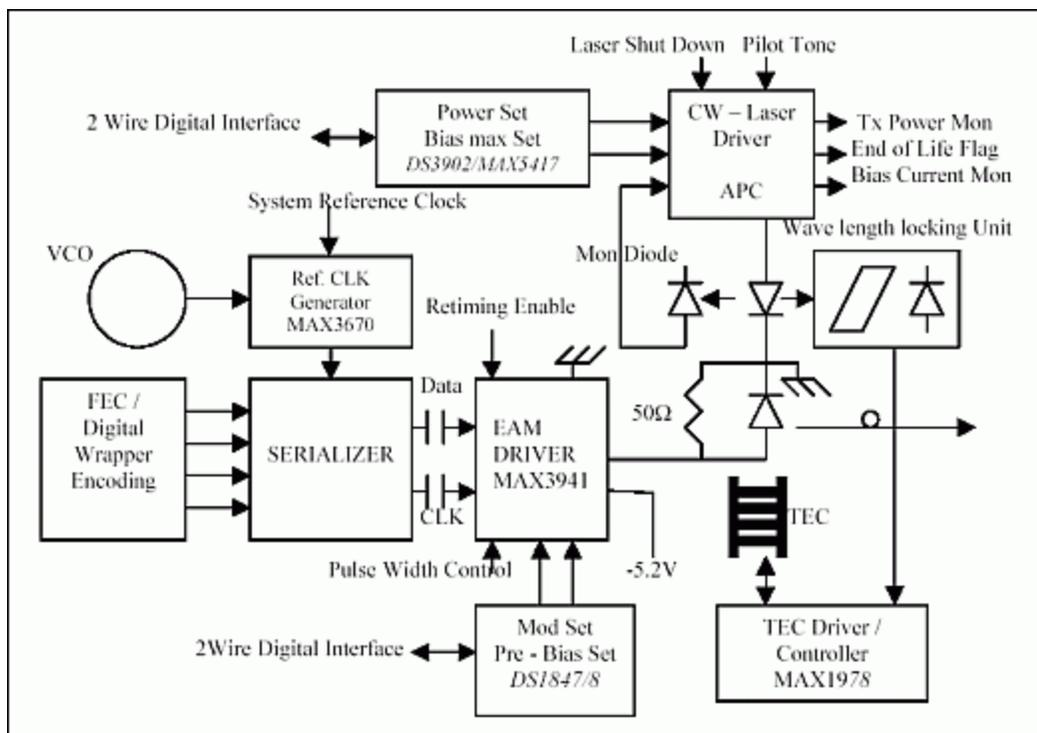
Figure 2. Example of a 10Gbps DWDM transmitter.
