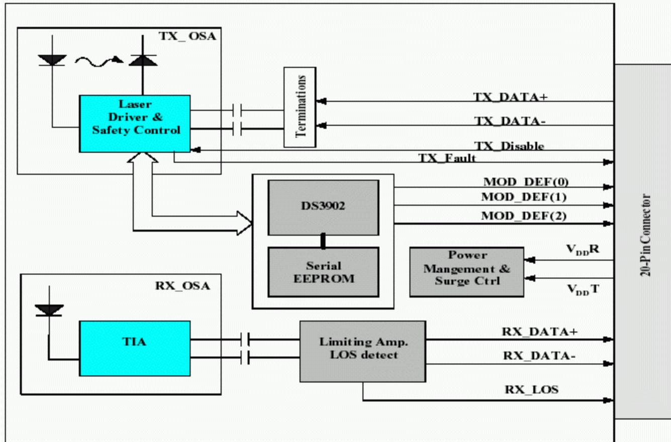
Figure 1. Typical optical module block diagram.
