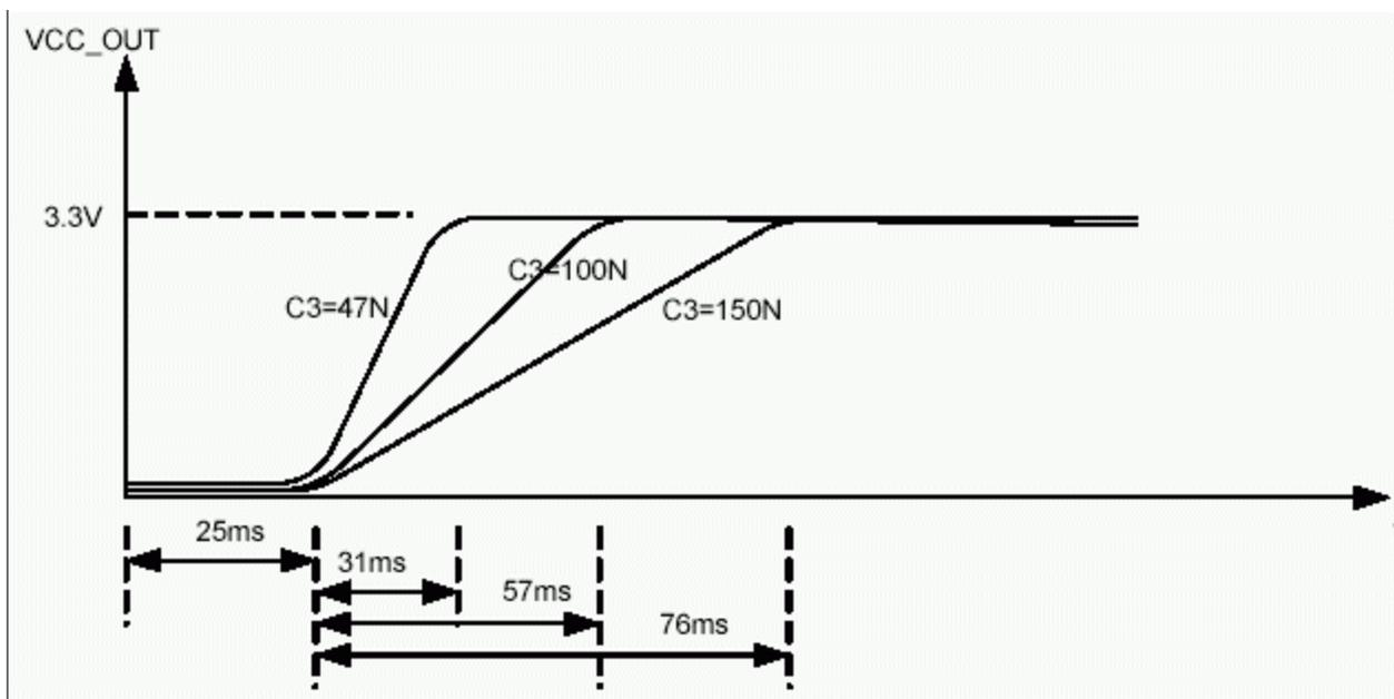
The above is response to a step-input voltage 0V to 3.3V. The current surge is well below the 360mA maximum current output with the component values given in the schematic.
