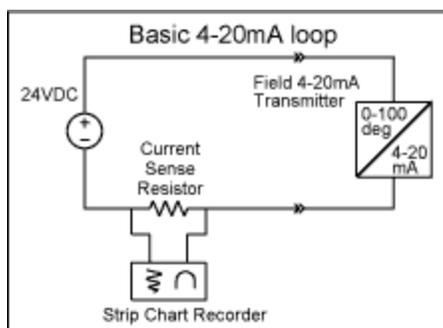
Figure 1. Basic architecture of a 4-20mA current loop.
