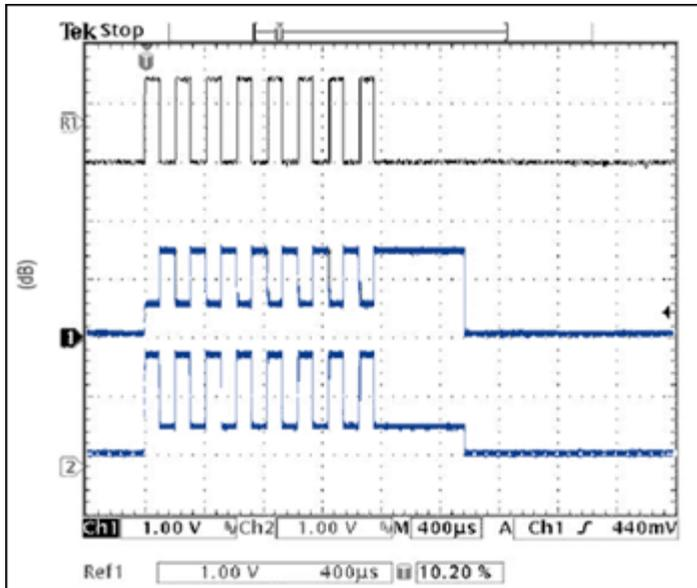
Figure 2. An input data byte causes the repeater to transmit the byte, then go to standby. Vertical scale is 1V per division; horizontal scale is 400µs per division.
