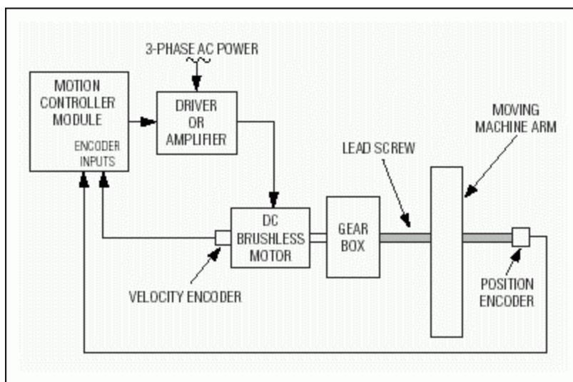
Figure 1. This DC brushless servo system uses quadrature optical encoders to provide velocity and position
