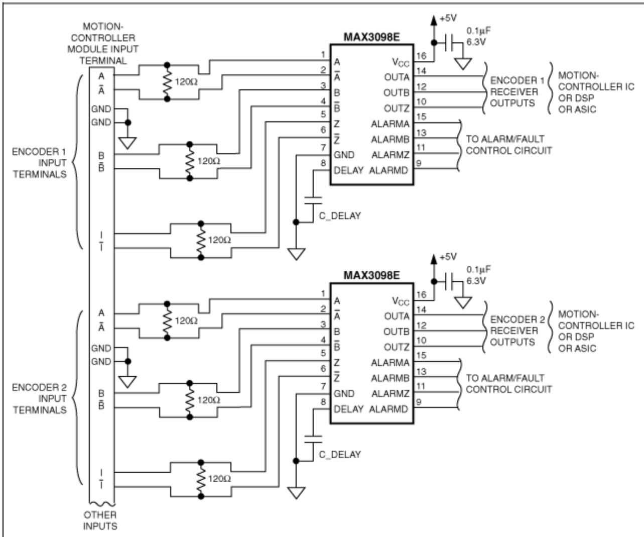
Figure 3. This circuit improves that of Figure 2 with detection of open, shorted, and intermediate faults, ESD protection on all encoder input lines, and delayed alarm/fault outputs.
