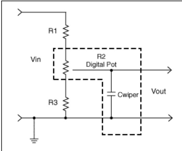
Figure 1. Typical Digital Potentiometer circuit configuration.
