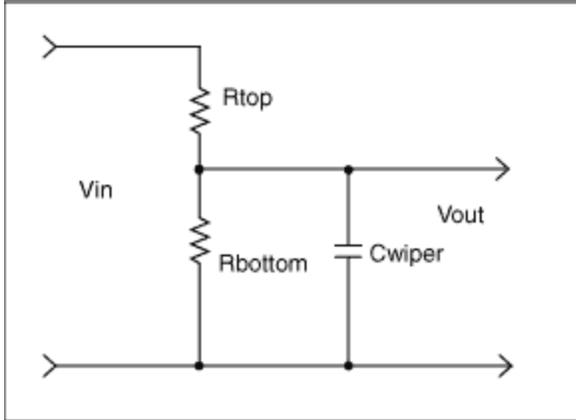
Figure 9. Circuit with the simplifications of Figures 7 and 8.
