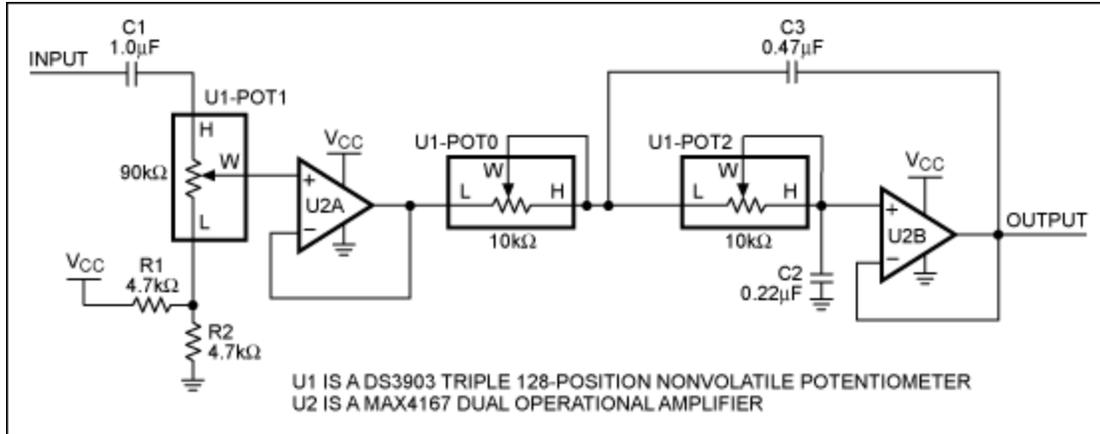
Figure 1. Audio range lowpass filter using a DS3903.
