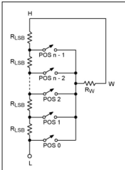
Figure 2. Digital potentiometer resistor model.
