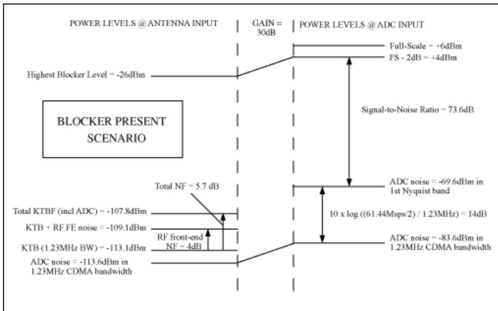
Figure 3. ADC noise contribution for blocker present.
