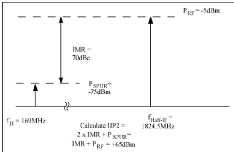
Figure 5. 2<sup>nd</sup> -order intercept calculation for signals referred to mixer input, IIP2.
