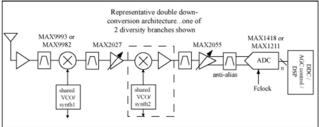
Figure 1. Subsampling receiver architecture.
