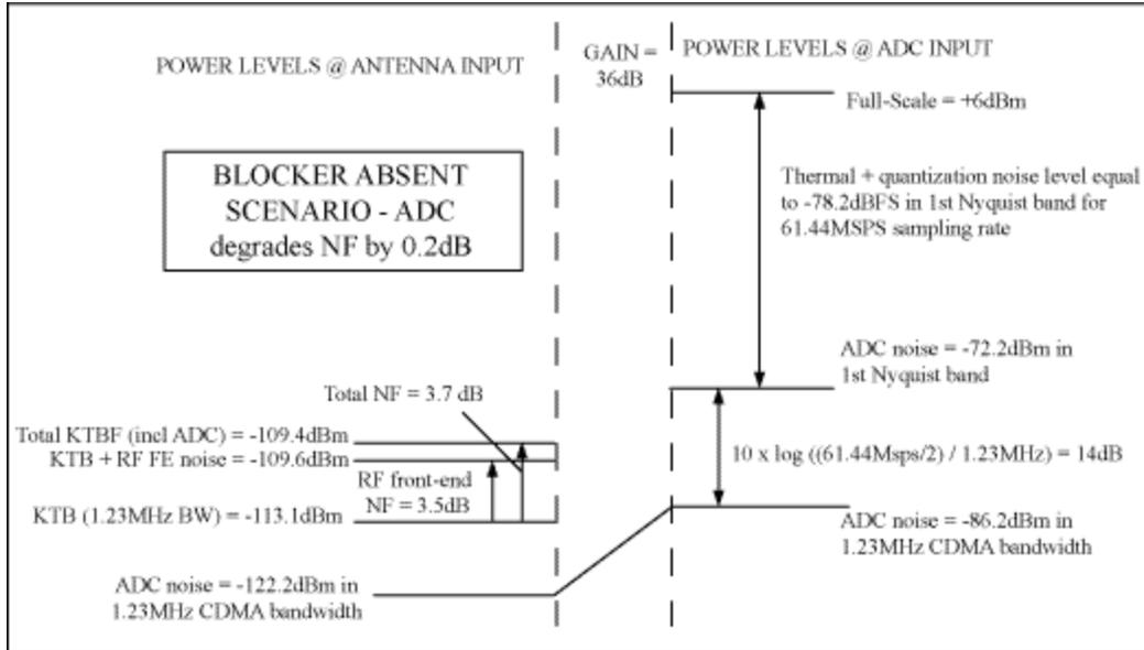
Figure 2. ADC noise contribution for no blocker.
