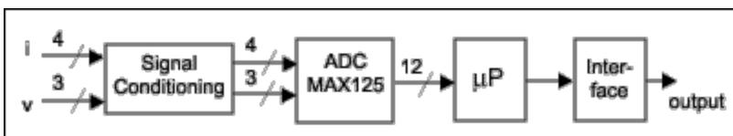
Figure 6. This simplified diagram shows the major blocks in a line-fault protector.
