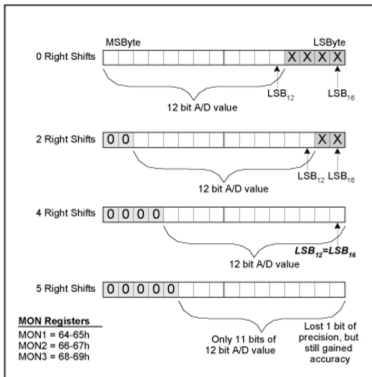
Figure 3. MON register right shifting examples.
