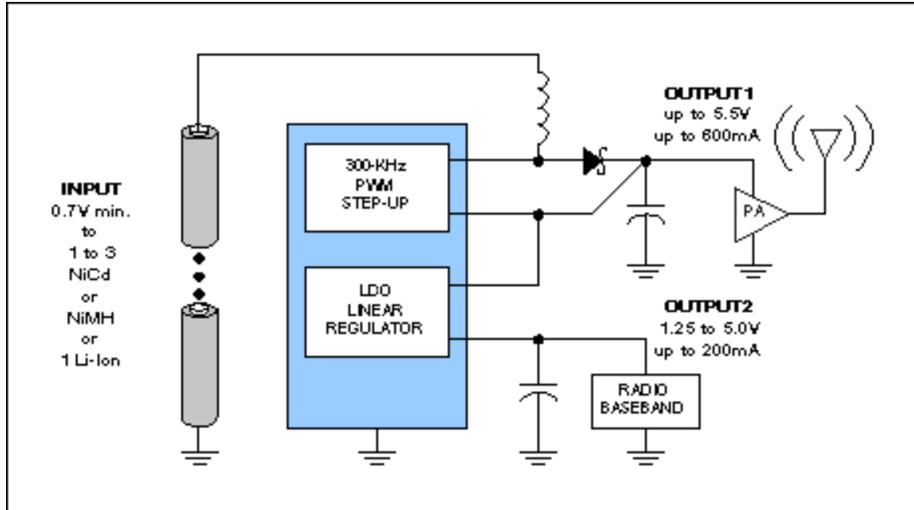
Figure 1. To provide high-efficiency boost and buck/boost outputs on the same chip, the MAX1705 and MAX1706 ICs integrate a PWM step-up DC-DC converter with a low-dropout (LDO) linear regulator. Designed for flexibility, these devices allow operation from a single Li+ cell or from batteries of one, two, or three NiCd, NiMH, or alkaline cells.
