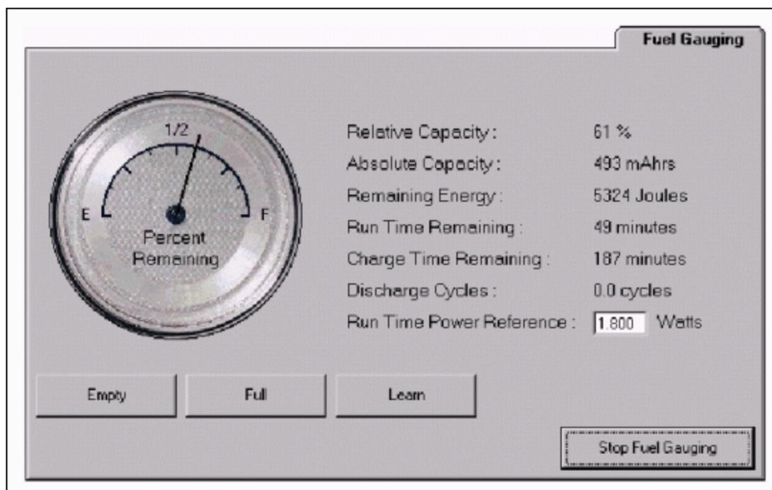
Figure 4. Fuel gauging tab of the evaluation software.
