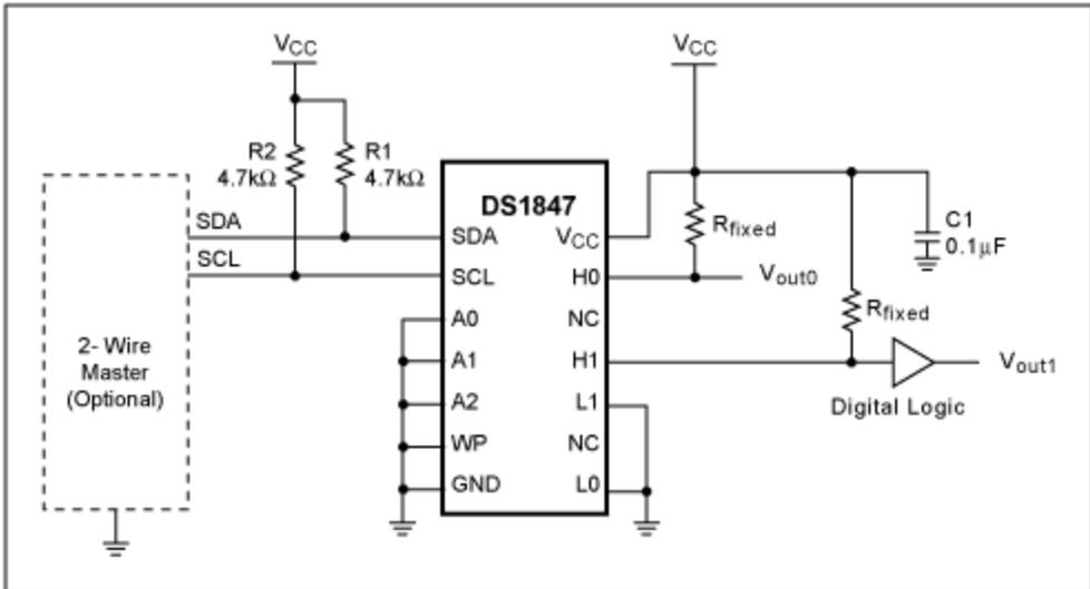
Figure 4. Voltage and digital outputs.
