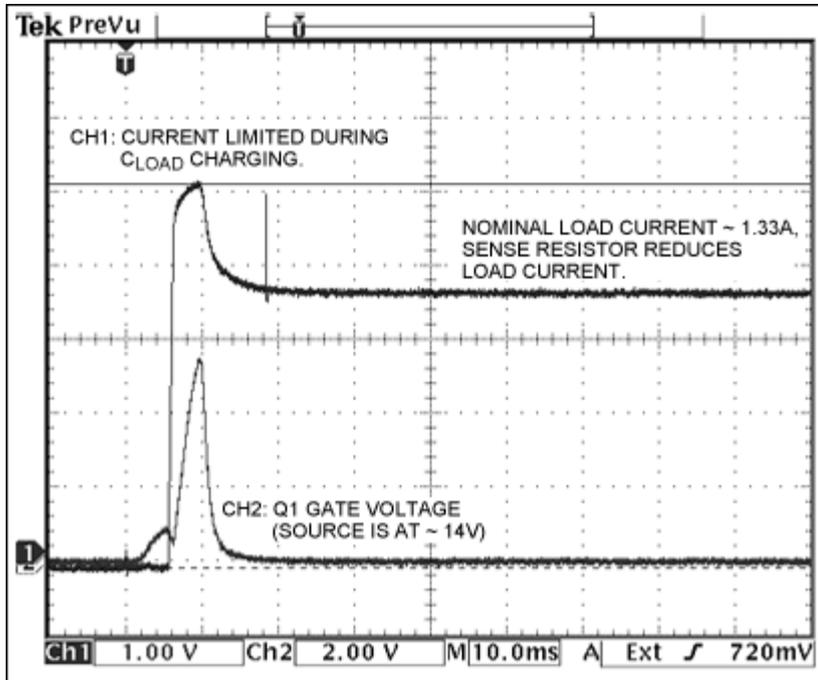
Figure 2b. CH1 is current; CH2 is Q2 gate voltage.
