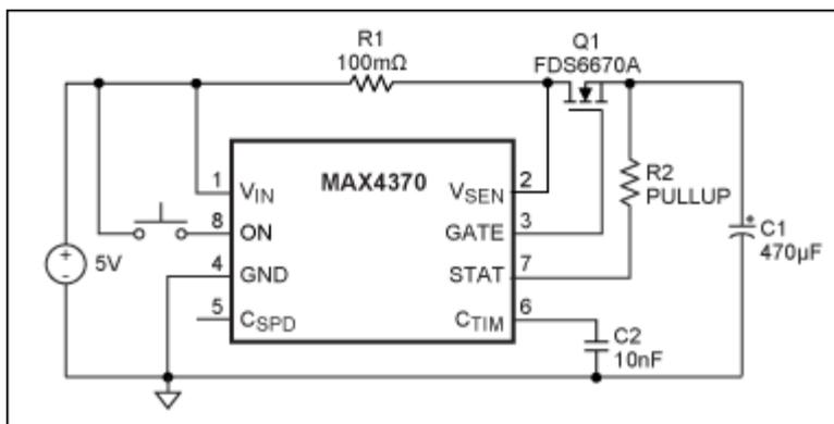
Figure 3a. An IC-based hot-swap circuit using the MAX4370 offers better accuracy and uses few components.
