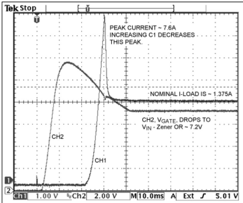
Figure 1b. CH1 is load current; CH2 is Q1 gate voltage.
