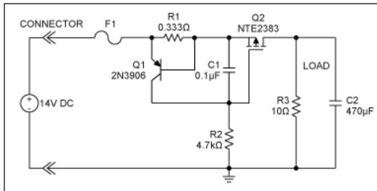
Figure 2a. Another hot-swap circuit implements current sensing and 2A limiting with a PNP transistor (Q1). This is illustrated by the turn-on waveforms in Figure 2b.
