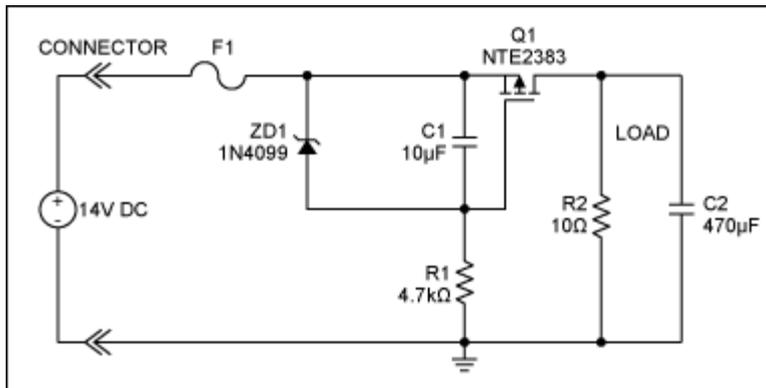
Figure 1a. A discrete "cap-zener-FET" hot-swap circuit uses the charge rate of C1 to control the turn-on of Q1. This is shown in the scope plot of Figure 1b.
