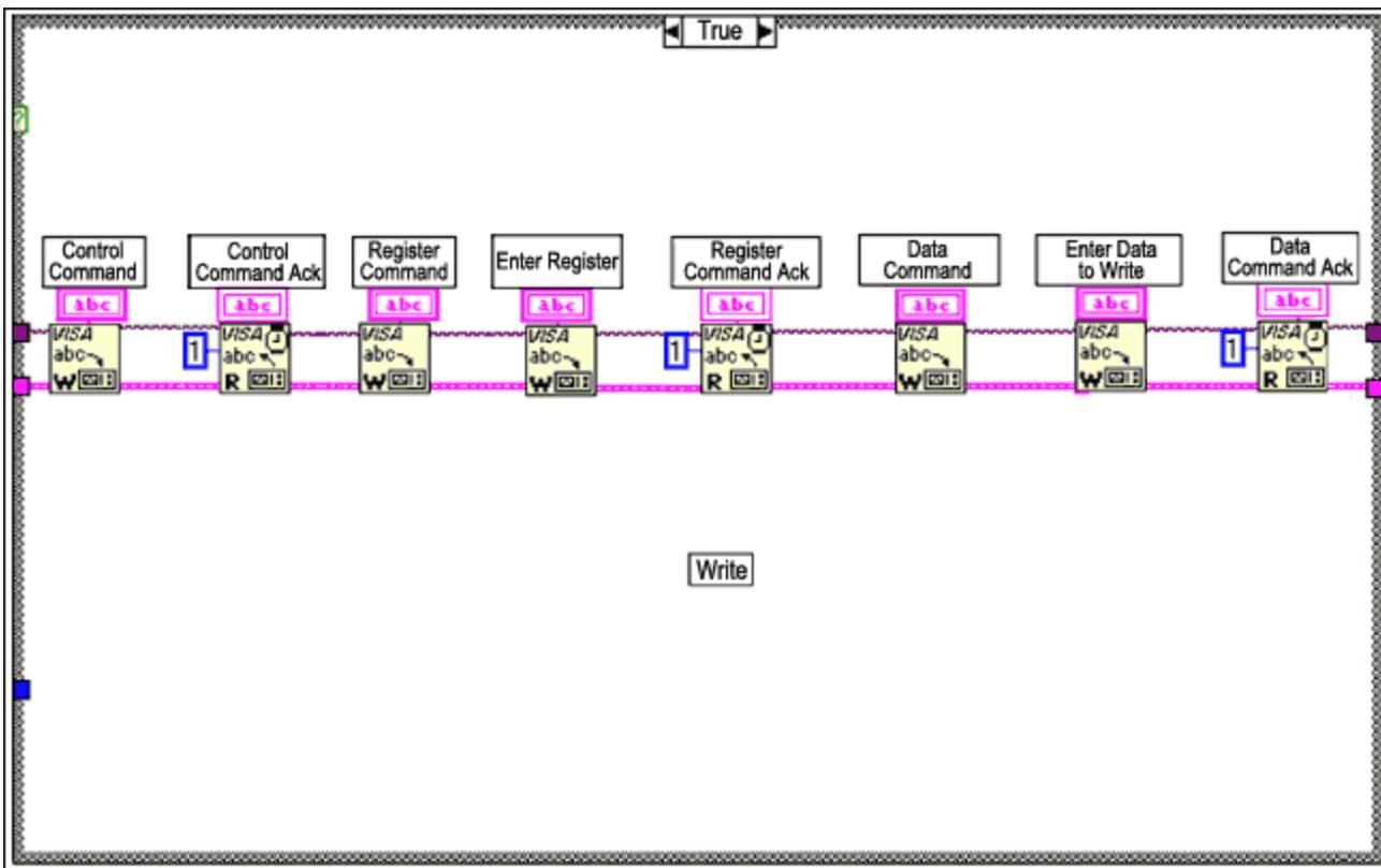
Figure 7. Serial Write.
