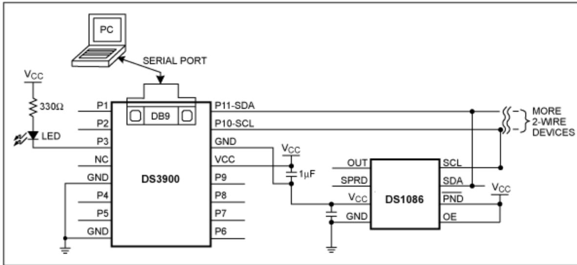
Figure 2. Typical Operating Circuit.
