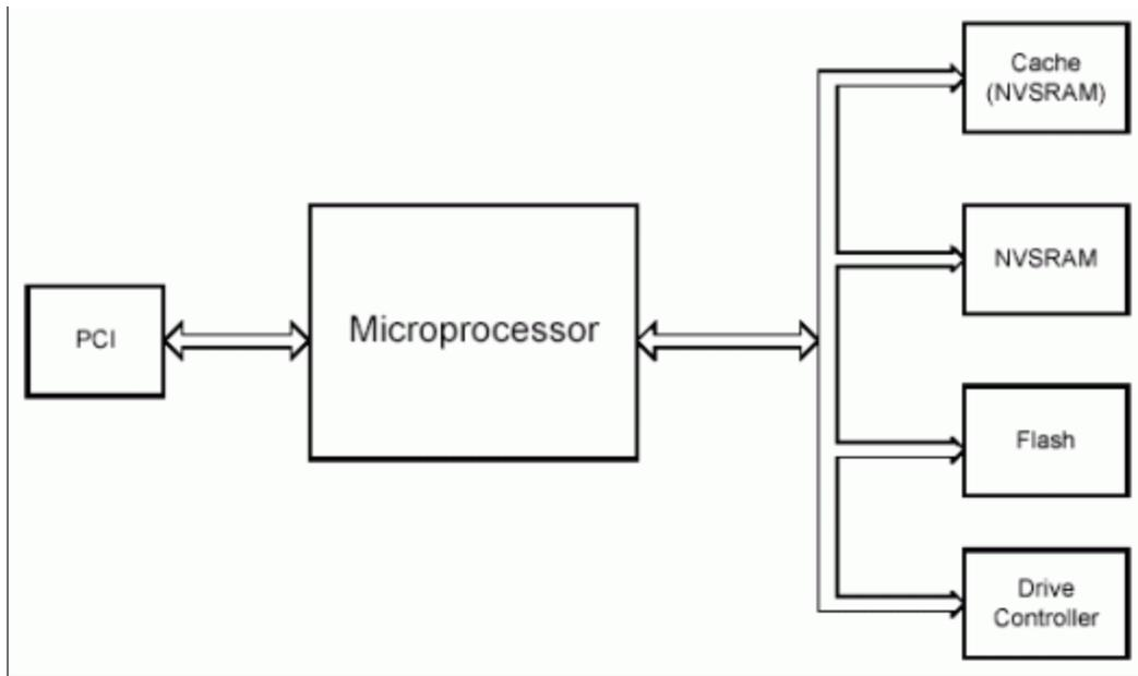
Figure 1. NV SRAMs in a RAID controller.
