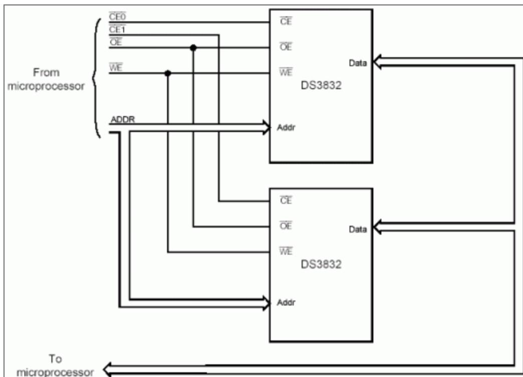
Figure 2. Connecting multiple NV SRAMs.
