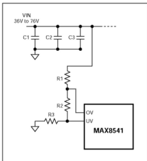
An alternate method used in the application circuits for setting the over-voltage and under-voltage trip points is demonstrated in **Figure 2**. Use 36.5kΩ for the bottom resistor (R3). R2 and R1 are calculated as follows:
