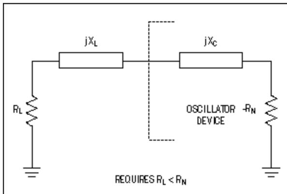
Figure 4. Reflection amplifier model.
