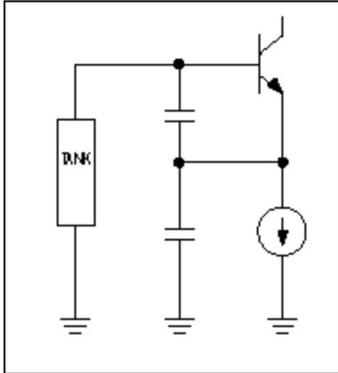
Figure 1. The basic Colpitts oscillator.
