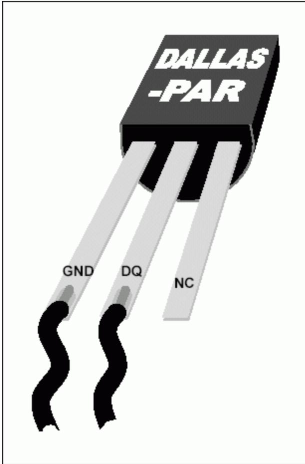
Figure 4. -PAR wiring configuration.
