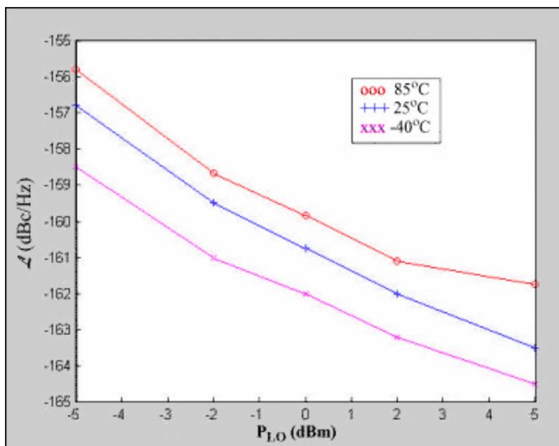
Figure 6. Local oscillator noise ( $\mathcal{A}$ ) in dBc/Hz versus input local oscillator drive power into MAX9982 as a function of temperature.
