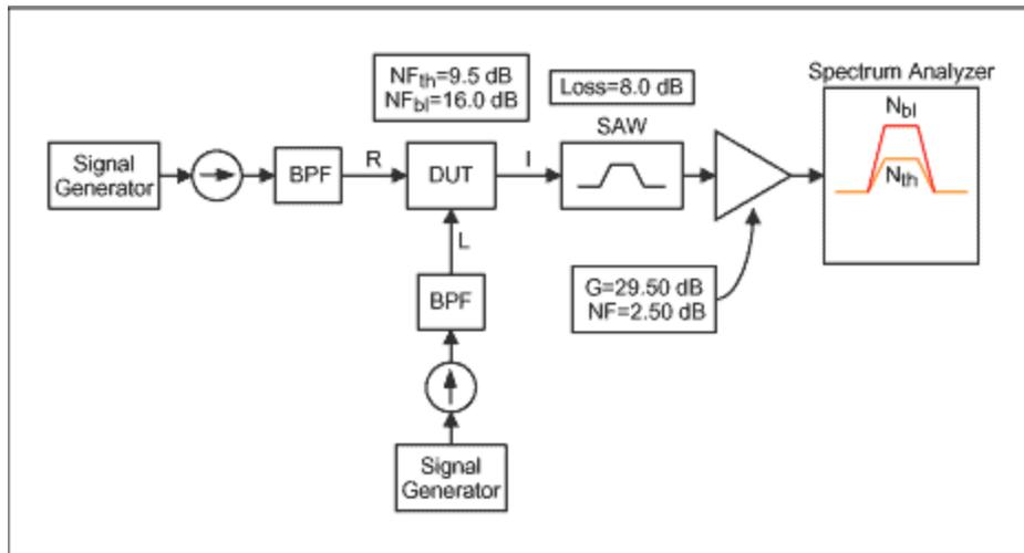
Figure 5. Experimental set-up to measure noise under blocking conditions and deducing  $\mathcal{A}$ .
