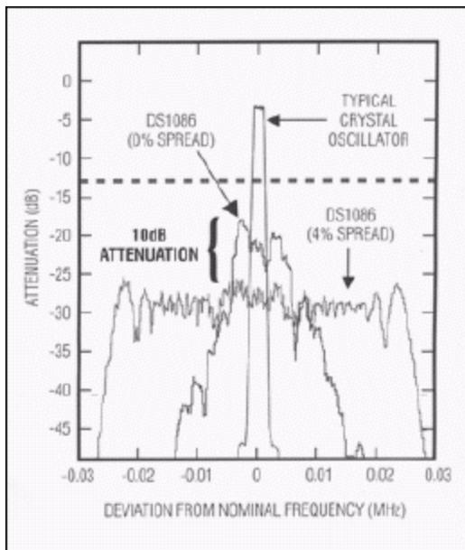
Figure 3. Clock spectrum dither comparison.
