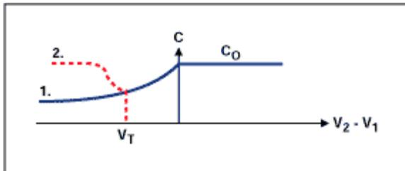
Figure 3. Variation of a capacitor with applied voltage.
