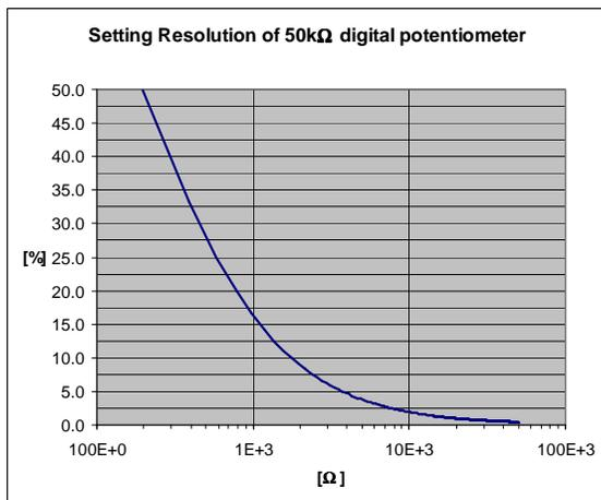
Figure 1. Setting resolution of 50kΩ digital potentiometer
