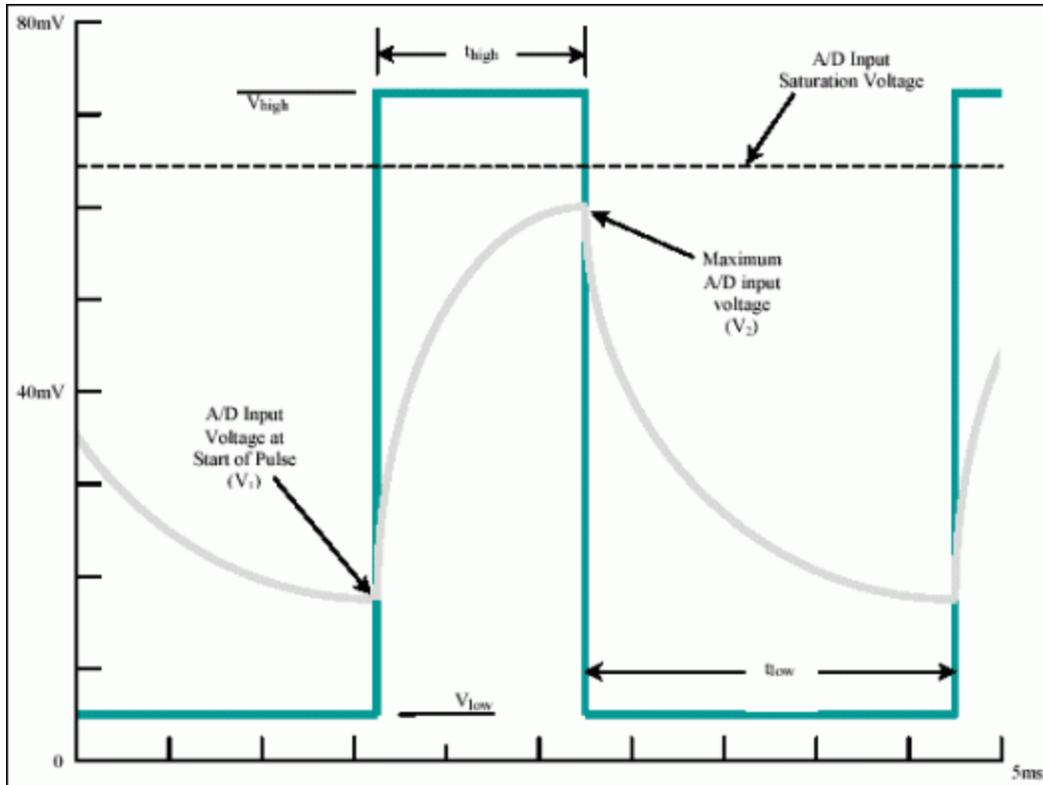
Figure 2. Filtered and unfiltered waveforms.
