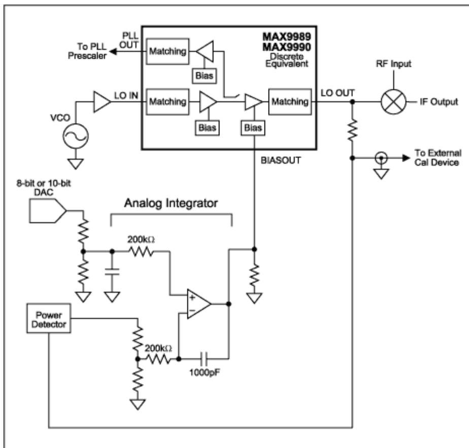
Figure 8. Analog closed loop control.
