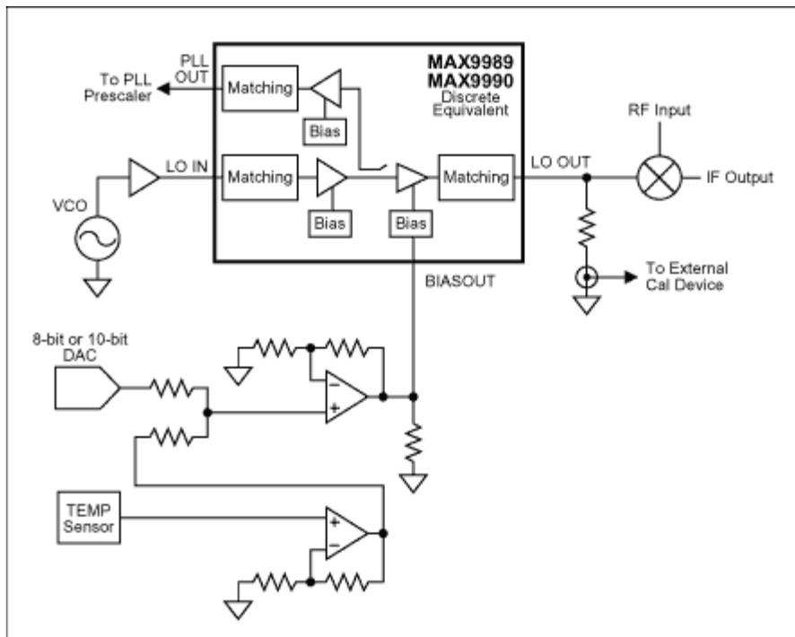
Figure 7. Temperature compensation using an analog technique.
