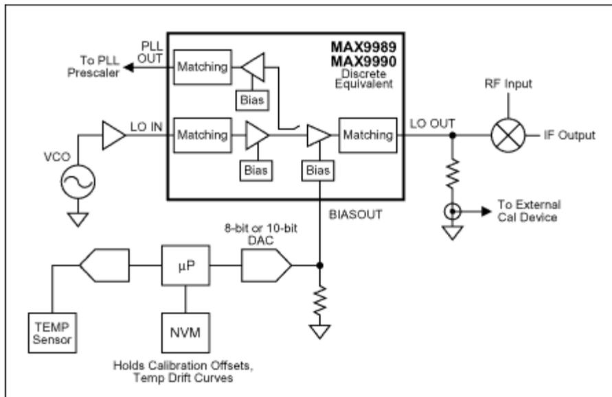
Figure 6. Temperature compensation using a digital technique.
