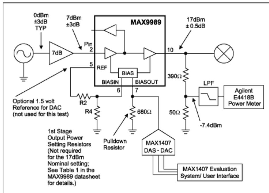
Figure 4. RF sense and DAC power control circuit for the MAX9989/MAX9990 (single output versions).
