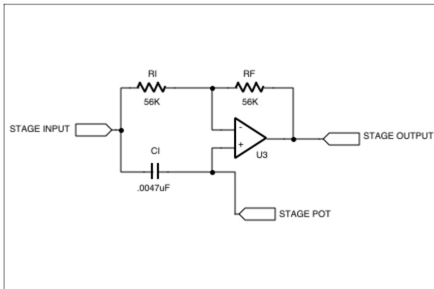
Four sections of the DS1806 are used to control the phase shift of each stage under microprocessor control. Note that two pot sections are left over, available perhaps for use as level controls.
