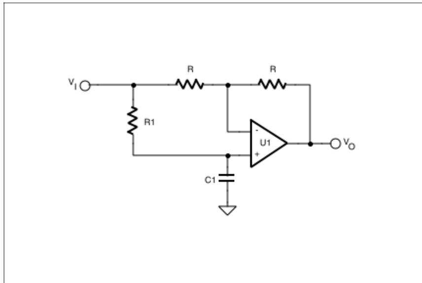
As the signal frequency varies from DC to infinity, the phase shift will vary from 0 to +180 degrees. You can also see that by varying R1, the phase shift at a given frequency will vary likewise. If the position of R1 and C1 are reversed, as in Figure 2, the transfer function becomes
