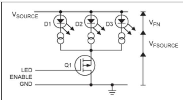
Figure 6. LED biasing with current sources.
