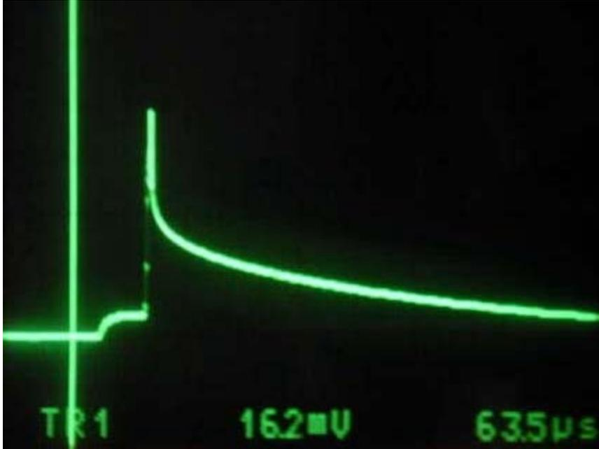
Figure 5. Clamp overshoot (at pulse output); horizontal scale = 50µS/div, vertical scale = 50mV/div, supply voltage = 4.5V, clamp overshoot = 162mV.
