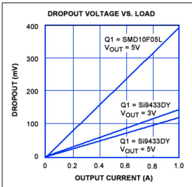
Figure 1. A p-channel MOSFET (Q1) allows this linear regulator to operate with  $V_{IN}$  to  $V_{OUT}$  differentials lower than 100mV.
