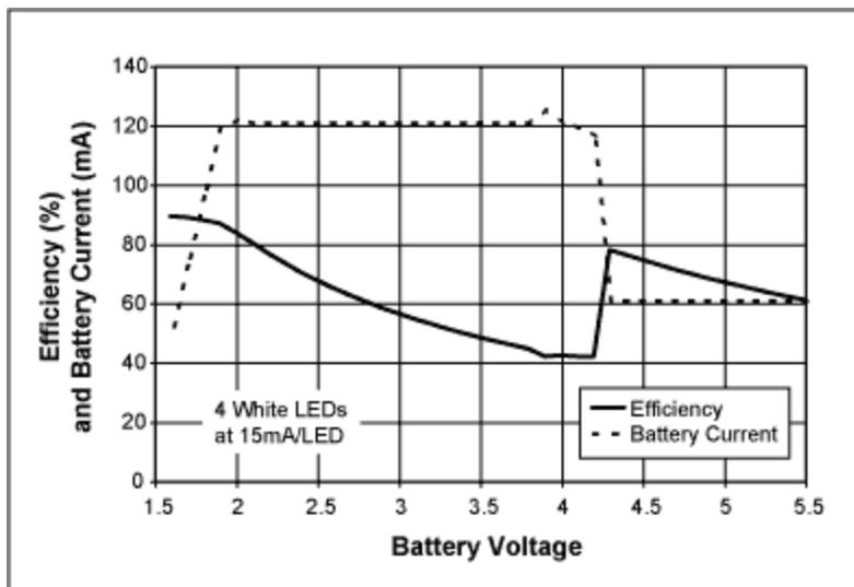
Figure 2. The efficiency and battery current for the circuit of figure 1 varies with battery voltage, especially when transitioning from 1x buck mode to 2x boost mode at approximately 4.25V input.
