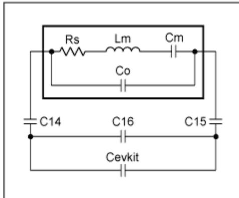
Figure 3. EVKit equivalent circuit.
