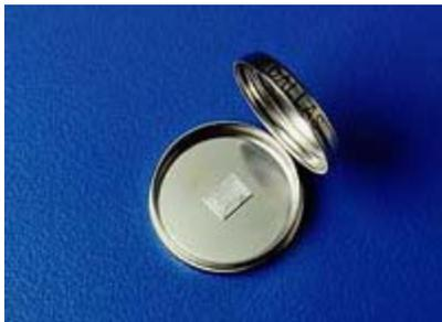
An iButton device uses its stainless steel 'can' as an electronic communications interface. Each can has a data contact, called the 'lid', and a ground contact, called the 'base'. Each of these contacts is connected to the silicon chip inside. The lid is the top of the can; the base forms the sides and the bottom of the can and includes a flange to simplify attaching the iButton device to just about anything. The two contacts are separated by a polypropylene grommet.
