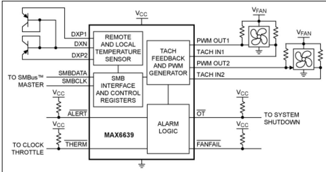
Figure 4. MAX6639 controlling two 4-wire fans. The MAX6639 measures two temperatures and can control fan RPM based on the measured temperature.
