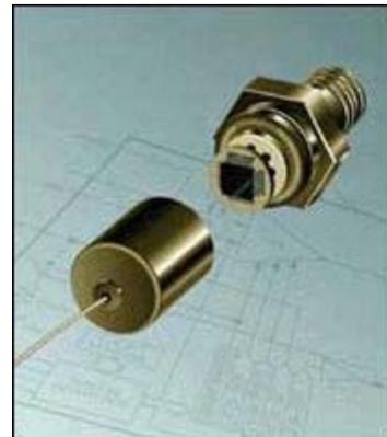
monocrystalline semiconductor (a piezoelectric effect) is substantially higher than that in standard strain gauges, whose resistance changes with geometrical changes in the structure. Conductivity in a doped semiconductor is influenced by a change (compression or stretching of the crystal grid) that can be produced by an extremely small mechanical deformation. As a result, the sensitivity of monocrystalline sensors is higher than that of most other types. Specific advantages are:
