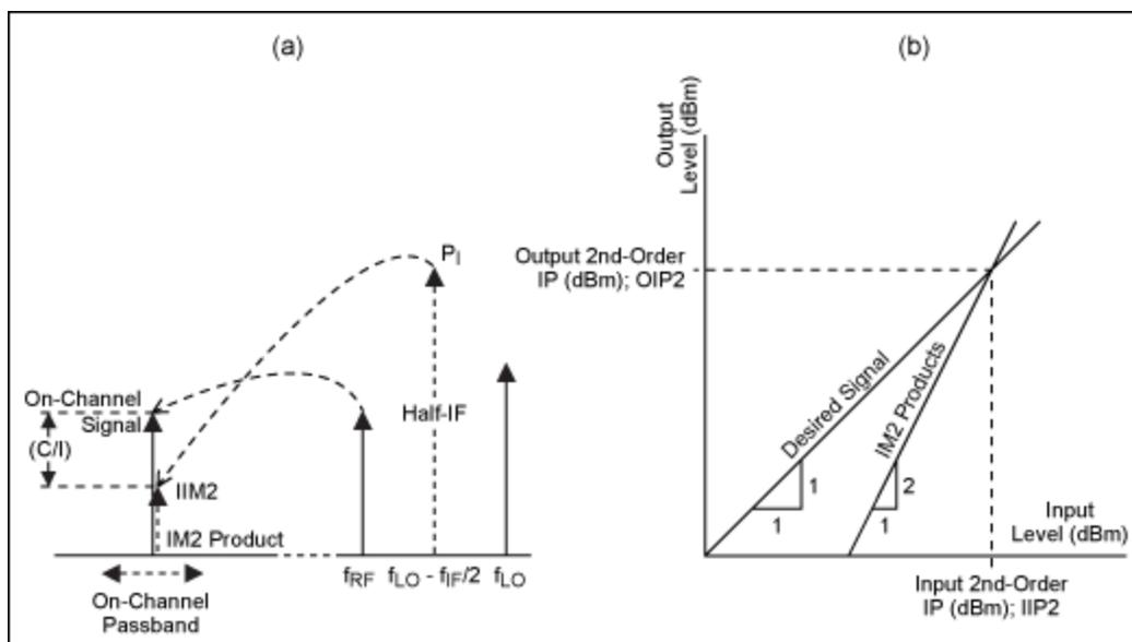
Figure 4. IM2 product as an in-band interferer due to half-IF spurious response (a), and second-order
