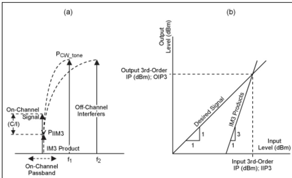
Figure 1. IM3 product as an in-band interferer due to two off-channel CW tones (a), and third-order intercept point (IP) definition (b).
