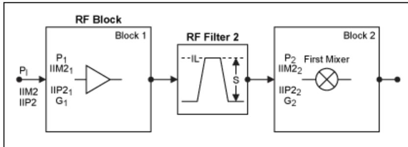
Figure 5. Block diagram for deriving the modified IP2 cascading equation, which incorporates the effect of adding RF selectivity (S) to the receiver's RF front-end stages at the half-IF spurious frequency. Power symbols are in dBm, and gain is in dB.
