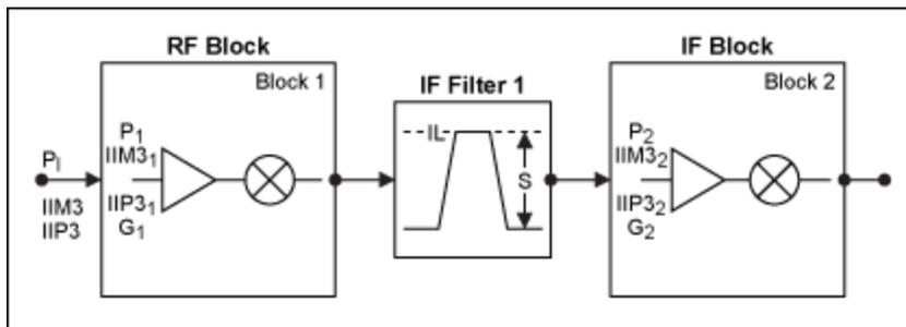
Figure 3. Block diagram for deriving the modified IP3 cascading equation. The equation incorporates the effect of adding selectivity ( $S$ ) to receiver stages at the two off-channel CW tones' frequencies. Power symbols are in dBm, and gain is in dB.
