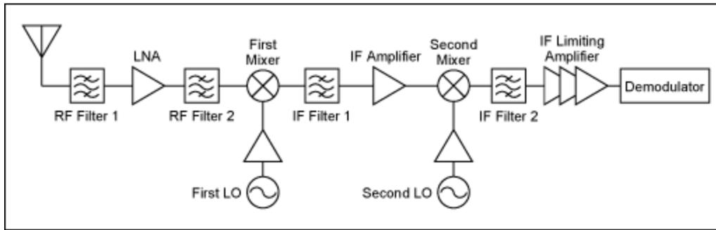
Figure 2. Conventional superheterodyne dual-conversion receiver.
