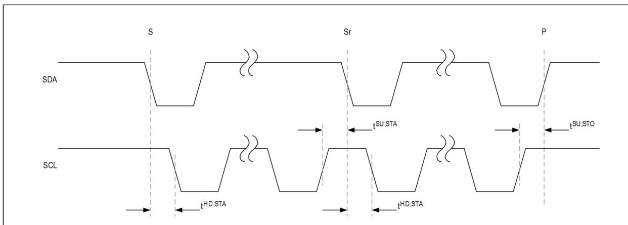
Figure 3. I<sup>2</sup>C START and STOP conditions.
