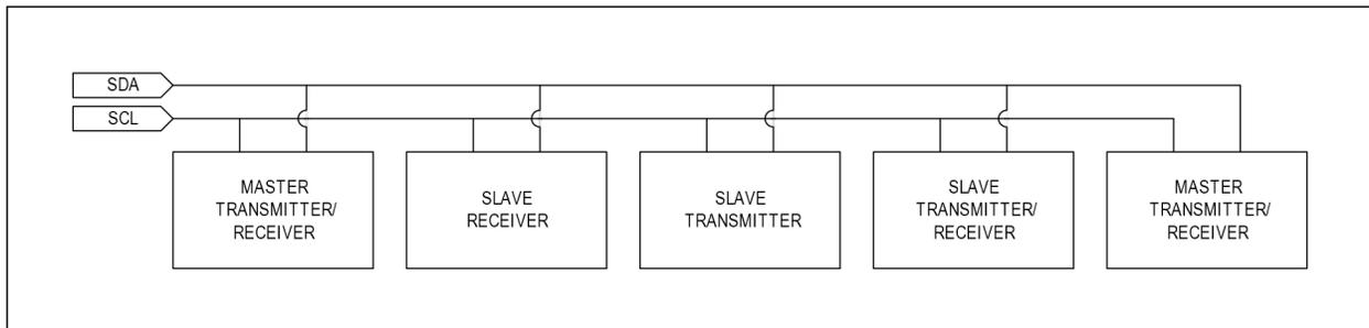
Figure 2. I<sup>2</sup>C system configuration.
