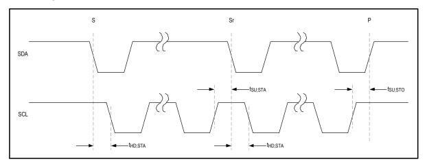
Figure 3. I<sup>2</sup>C START and STOP conditions.
