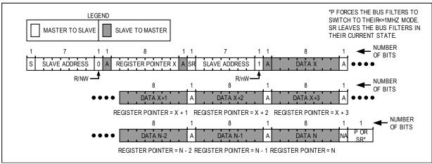
Figure 8. Reading from multiple registers.
