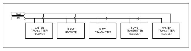
Figure 2. I<sup>2</sup>C system configuration.
