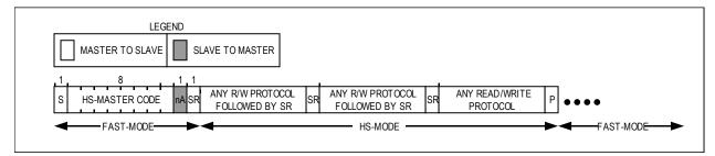
Figure 9. Engaging high-speed mode.
