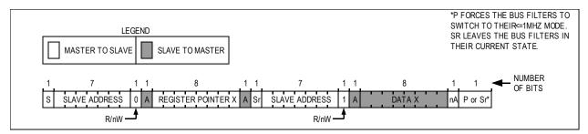
Figure 7. Reading from a single register.
