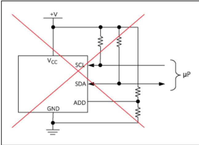
Figure 3. Do not use pullup or pulldown resistors on a "No Connection" pin configuration.
