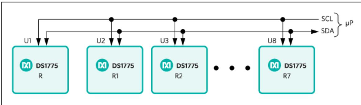
Figure 4. Ordering-defined addressing is implemented in the DS1775 and MAX6697 temperature sensors.
