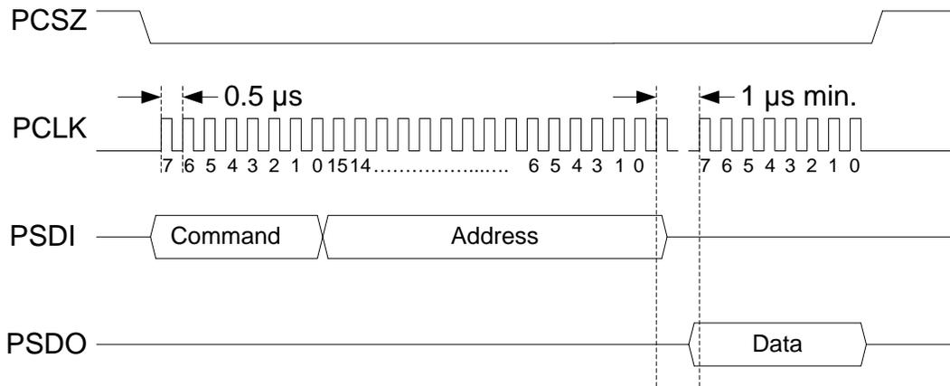
Figure 2: SPI Slave Port: Read Operation with Gap
