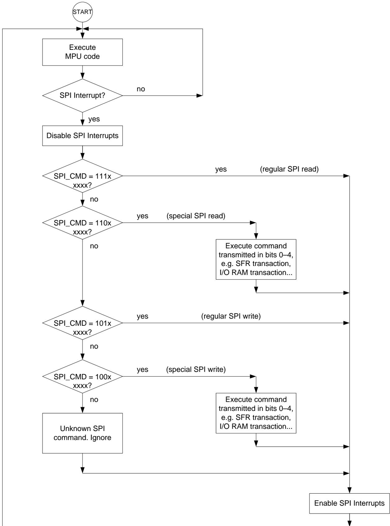
Figure 6: Interrupt Processing Flow Chart
