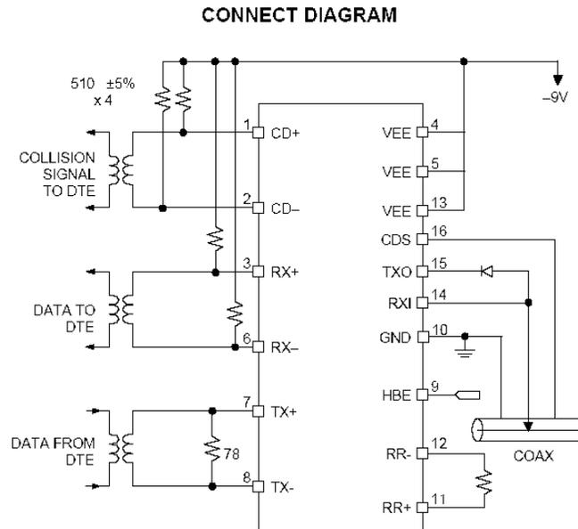
The CD+/- termination resistor may be increased to  $1.5K\Omega$  to save power. Refer to the CD+/- pin description in the data sheet for specific information.
