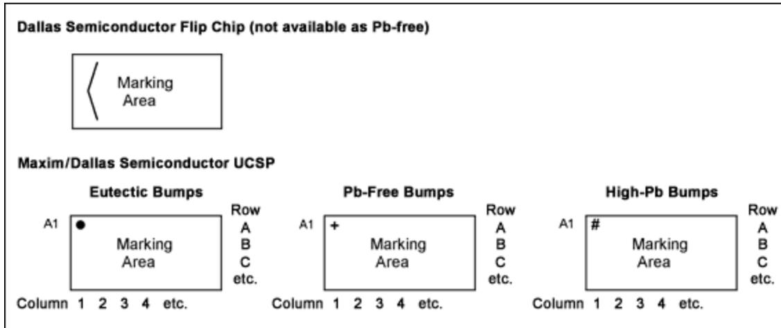
Figure 4. Flip chip and UCSP marking templates.
