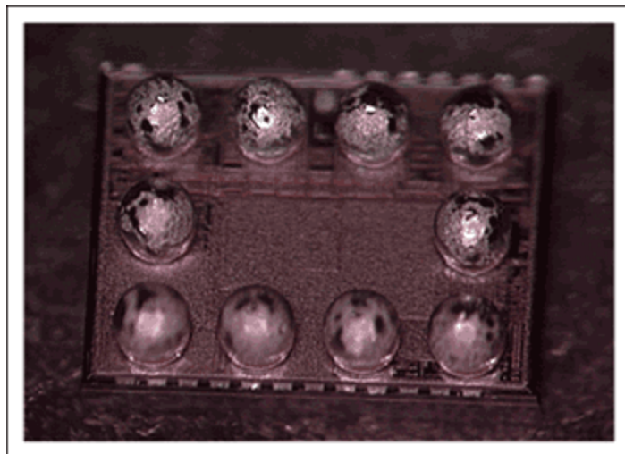
Figure 2. A 12-bump chip-scale package, 3 x 4 bumps, with 2 bump locations not populated.
