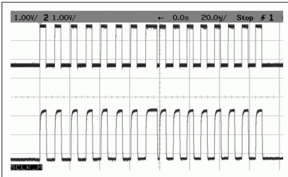
Figure 7. The SPI SCLK signal on both sides of the isolated interface. Top: ISOV<sub>CC</sub> = 8.3V, ISOGND = 5V. Bottom: Powered by USB: V<sub>CC</sub> = 3.3V, GND = 0V.
