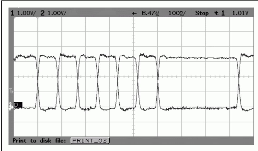
Figure 2. This scope trace shows the USB D+ and D- signals (site 1 in Figure 1) at the beginning of a packet. The 83ns bit time and close matching of rise/fall times make it difficult to maintain signal fidelity through optical isolators. D+ and D- are bidirectional, further complicating the isolation.
