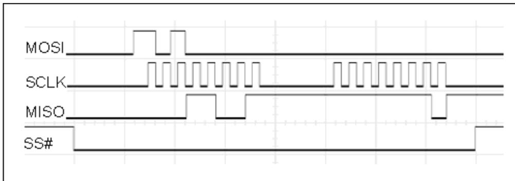
*Figure 3. An SPI interface operating in mode (0,0). The same interface can operate in mode (1,1) if the SCLK signal is made active-low (quiescent state is high). These low-frequency signals are easy to optically isolate.*
