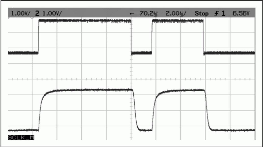
Figure 8. SCK isolated (top) and at the MAX342E (bottom), shown with expanded scale.
