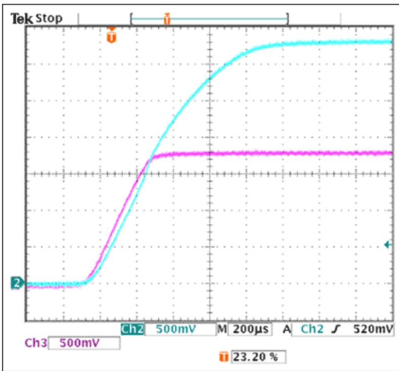
*Figure 2. Scope photo of output voltages in the open-loop tracking architecture of Figure 1, as controlled by the MAX6819 system-management device.*
