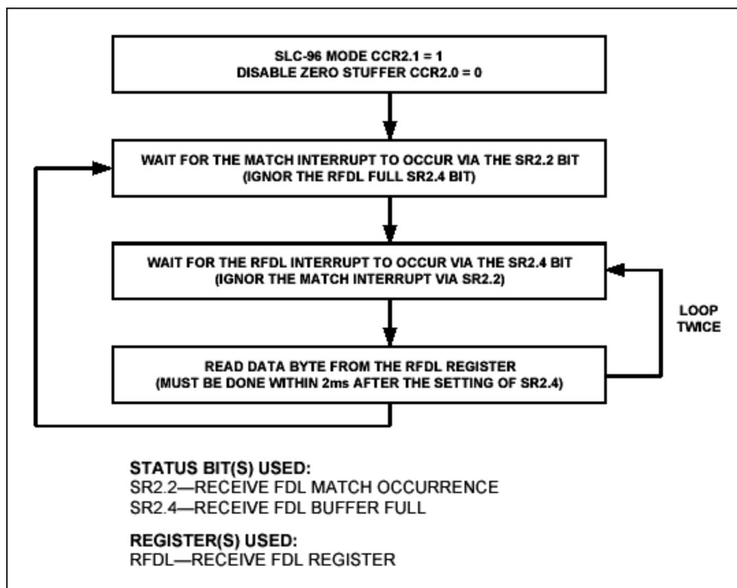
Figure 1. SLC-96 Message field extraction via RFDL.
