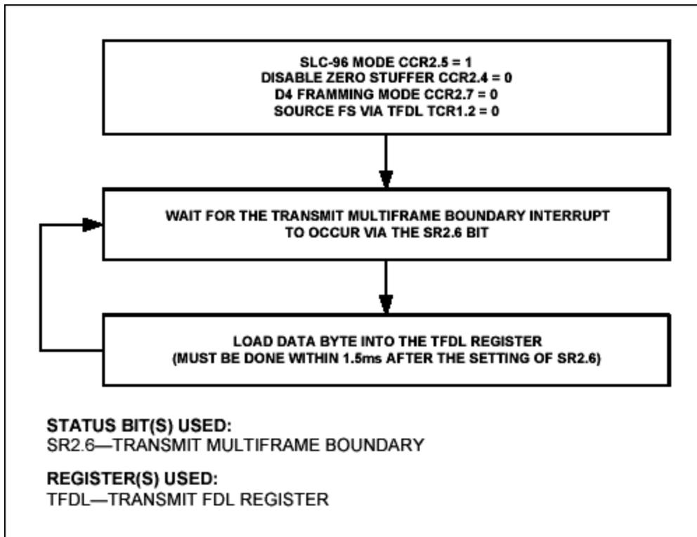
Figure 3. SLC-96 Message field insertion via TFDL.
