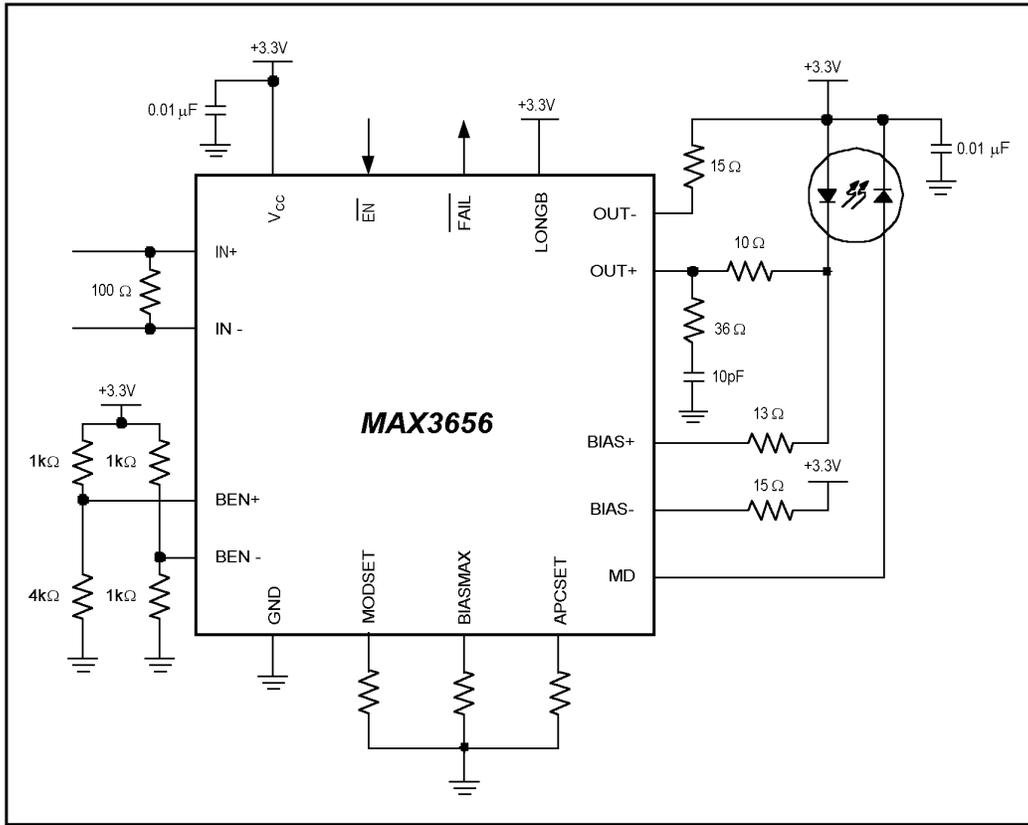
Figure 1. Application Circuit for the MAX3656
