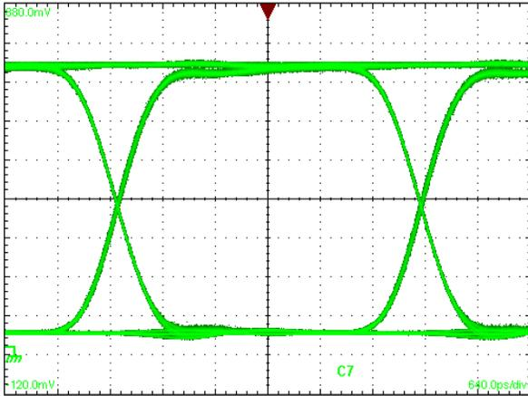
Figure 11. MAX3656 optical eye with  $2^{31}-1$  PRBS at 270Mbps.
